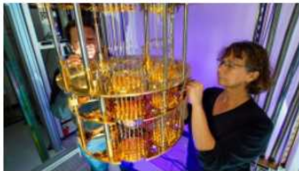
Jeanette Roberts of Intel adjusts a dilution refrigerator, which creates the ideal environment for qubit performance, at Intel Labs' Hillsboro, Oregon, campus. (Image by Walden Kirsch/Intel Corporation.)
